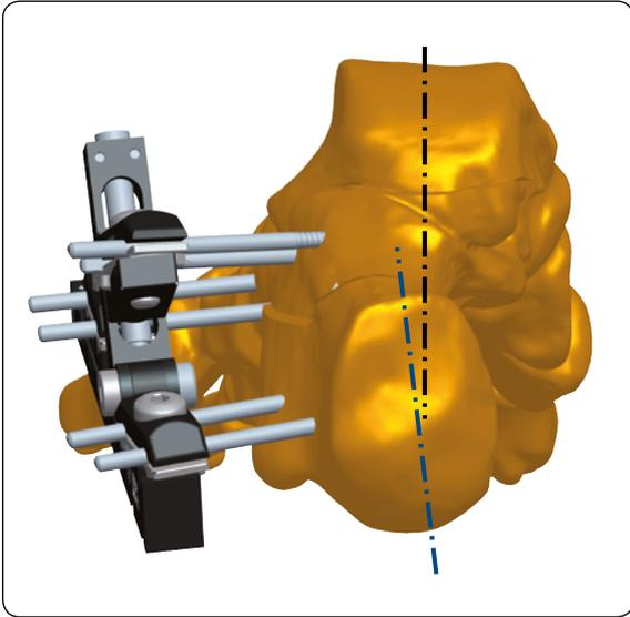
At this stage, when applying the pins at the level of the posterior or anterior calcaneal apophysis, it is possible to correct the varus-valgus deformity of the calcaneal body, by inserting the pin at an angle through the clamp that acts as a template. This angle can be captured by the pin clamp's swivel head.
