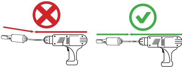
**Avoid toggling or bending the screw once inserted.**
